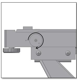
Figure 3. Turn power ON by rotating potentiometer.
