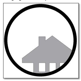
**3.1.** A distant object is centered at the telescope's field of view. In this example we have a house with a chimney. The chimney is the reference point to place at the center of the field of view. We first look through the telescope with the lowest magnification possible, so we have the widest field of view.
