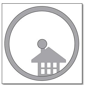
**3.3.** After playing with the two findercope thumbscrews and some trial and error, we get the finderscope red dot close to the center (in this case the chimney). The finderscope is now ready to use!
