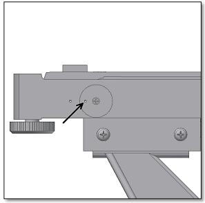
Figure 8. Turn potentiometer OFF.
