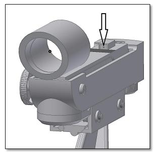
Figure 4. Red-dot lights up when ON.
