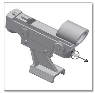
Figure 2. Remove plastic protection.
